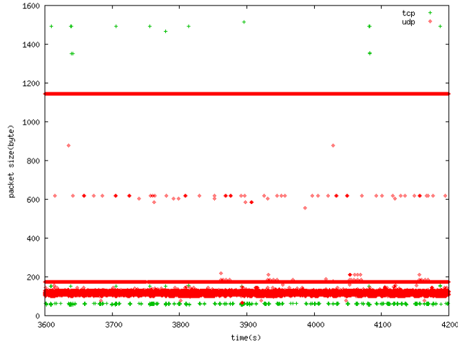
Fig. 2. Packet Size Distribution per Bearing Protocol
