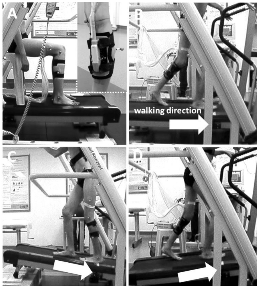
Fig. 4-1 Test conditions: A) seated rest measurement and ultrasound probe placement, B-D) treadmill walking for B) flat-forward, C) -12% backward-downhill slope and D) +12% uphill slope.
