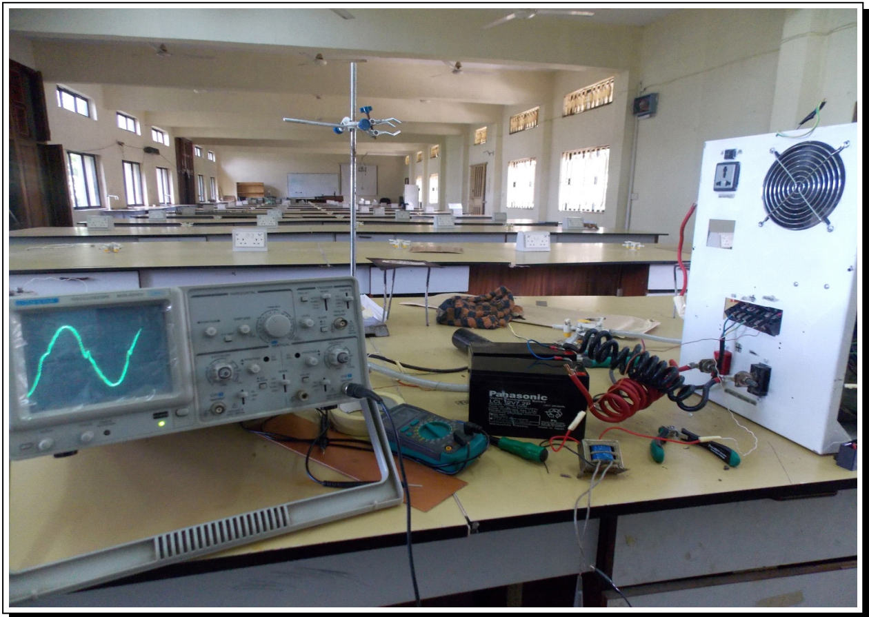
Figure 4. Sine wave obtained from PWM
