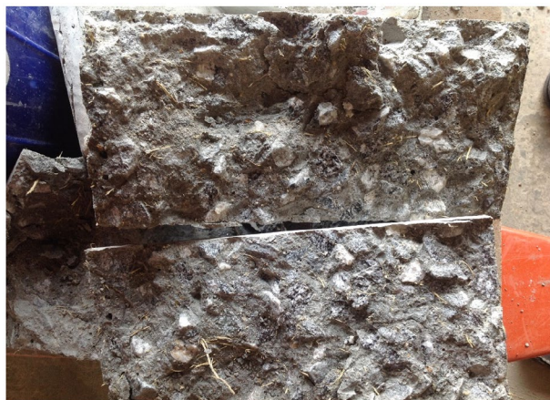
Figure 12. Ma-fiber concrete cylinder after splitting-tensile test.
