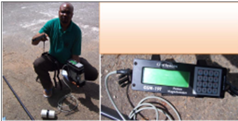
Fig. 2a. Portable magnetometer for ground magnetic survey
