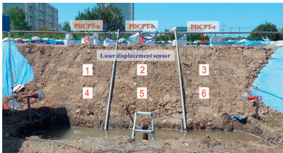
Fig. 6. Location of sampling points, laser displacement sensors and portable dynamic cone penetration tests (PDCPTs) on the landslide dam in Experiment 2.
