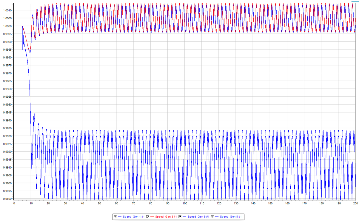
6.3- 10: Microgrid generator speed response in the fault situation after 33.3% load increase.
