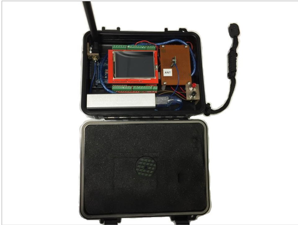
Figure 21 - Final Transmitter Experimental Apparatus
