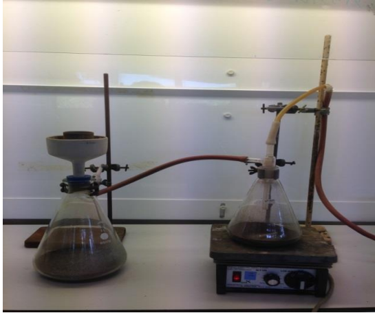
Figure 3.1 Separation of different soils components (a), and Extraction of soil and coarse mineral materials (b).
