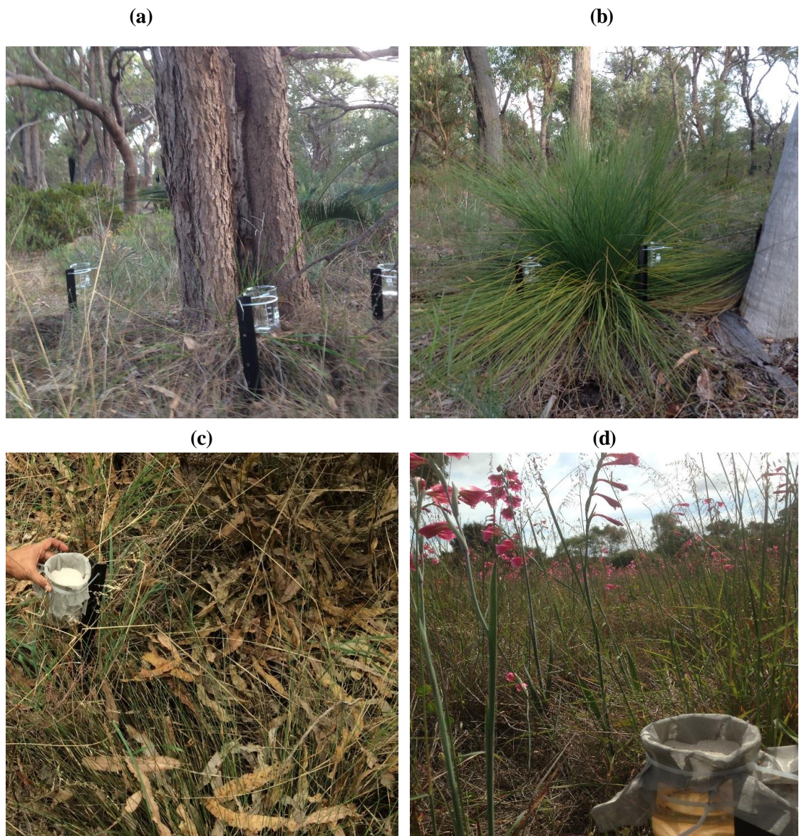
Figure 2.3 Capturing exudate under the canopies in the mounted glass beakers and aluminum mesh fitted on top of the beakers.
