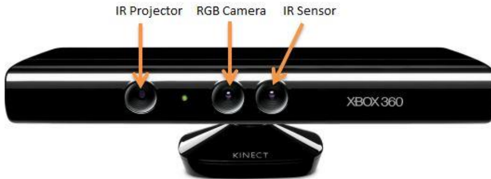
Figure 2 - Microsoft Kinect with the infrared projector, the RGB Camera and infrared sensor highlighted. 1
