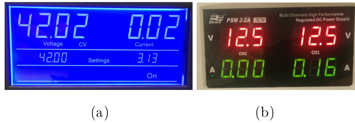
Figure 7.8: a) uMDC current consumption. b) MDC current consumption.
