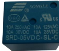
Figura 21 - EMR Songle modelo SRD-05VDC-SL-C.
