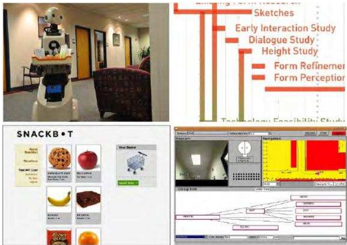
Figure 7. The Snackbot, a product service system to foster healthy snacking in an organization. Upper left: the robot. Upper right: The service design. Lower left: Web site for placing snack orders. Lower right: Dialogue system for interaction with customers.
