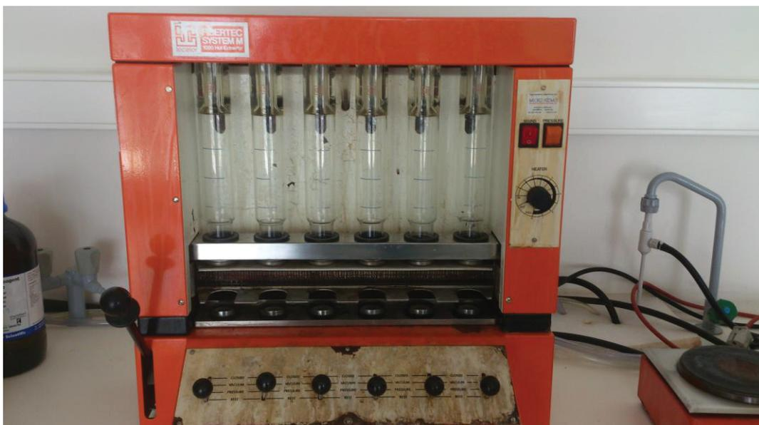
Figura 12 – Extrator Fibertec
