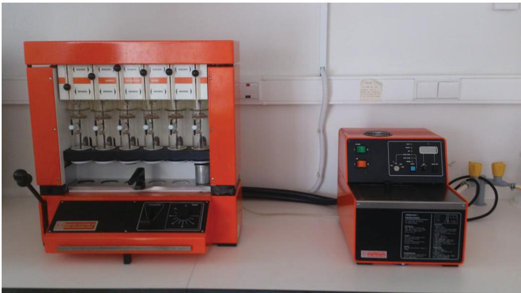
Figura 9 – Extrator Soxtec System HT
