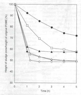
Fig. 3. Effect of Zeolite on settleability of POME. Symbols represent; control (●); 5g/L(□); 10g/L(◊); 30g/L (△); 60g/L (▲); 100g/L (◊)
