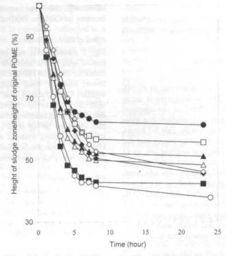
Fig. 2. Effect of Ferric chloride (FeCl.) on settleability of POME. Symbols represent; control (●); Ig/L(□); 2g/L(▲); 3g/L (■); 4g/L (△); 5g/L (◊); 6g/L (◊); 10g/L (0).
