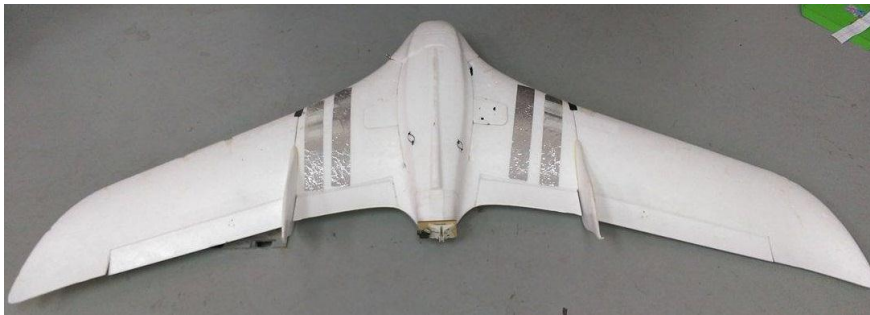
Figure 3. FX79 fixed wing with 2 m wingspan
