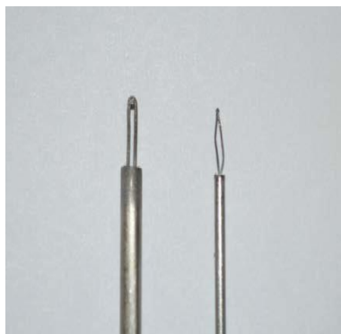
Figure 4. Baseline TC (1/8 inch) and smaller TC (1/16 inch) [20]
