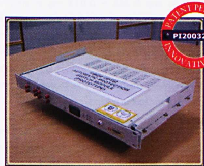
Automatic Protection Switch
