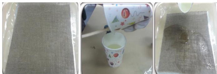
Figure 2. Specimen preparation for epoxy mixture.
