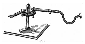
Figure 1 Bell's instrument for observing the photothermal effect. (http://fys.kuleuven.be/atf/Research\_themes/rt\_photoacoustic/rt\_photo\_pha)
