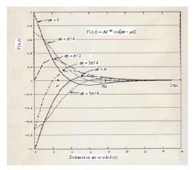
Figure 2 The profile of thermal wave as time progresses (or as phase  $\omega t$  changes)
