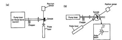
Figure 8 Photothermal Beam Deflection method (a) transverse, (b) collinear. (Jackson et al, 1980)
