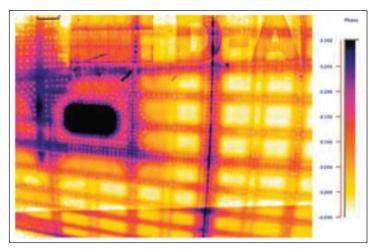
Figure 19 Fuselage inspection of a Boeing 737 using lock-in thermography shows the skin lap joints, stringers, doublers, and rivets. This image shows no defects. The frame station and the frame Tithe window appear in a darker color, an indication that they are made out of thicker material. (Vision Systems Design)
