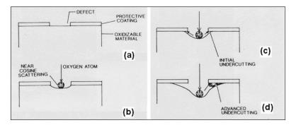
Figure 16 A possible scenario for undercutting of a defect coating in an ATOX environment. (Banks and Rutledge, 1988)
