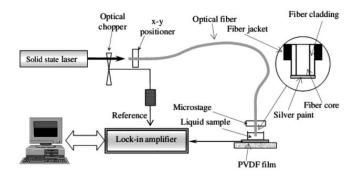
Figure 25 Schematic diagram of FO-TWRC technique. (Azmi et al., 2007)
