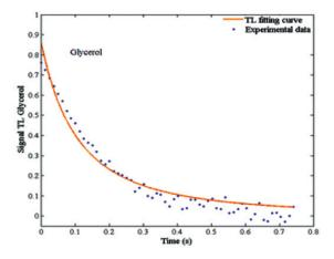
Figure 27 The thermal lens signal obtained by pulsed excitation. (Reza et al, 2012)
