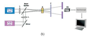
Figure 7 Schematic diagram of Thermal lens experimental set up using (a) CW excitation beam (Reza et al, 2011), (b) pulsed excitation beam. (L = lens, S = sample; F = filter; PD = photodiode detector)(Reza et al, 2012).
