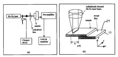
Figure 21 Experimental setup. (Azmi et al., 2002)
