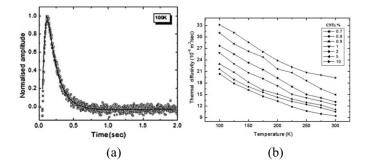
**Figure 26** (a) The transient signal by PVDF detector at the back of sample after photoflashing (b) The thermal diffusivity curves of sample at various temperature. (Moksin et al, 2013)
