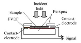
Figure 6 Schematic diagram of sample-PVDF holder
