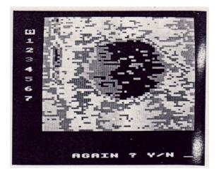
Figure 14 Phase image of a subsurface defect in an opaque sample with modulation frequency 100 Hz. (Kirkbright et al, 1984)
