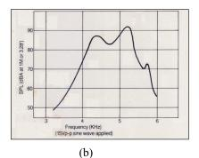
**Figure 4** Electret microphone (a) and its typical response (b)
