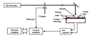
Figure 22 Schematic diagram of pyroelectric experimental setup. (Azmi et al, 2004)
