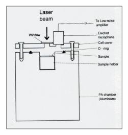
Figure 5 The small volume PA cell
