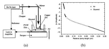
**Figure 23** (a) Schematic diagram of the experimental setup. (b) The amplitude of the pyroelectric signal on the cavity length for the two layer fluids: air and glycerol. The solid lines are the best-fit results of the experimental data. (Azmi et al., 2005)
