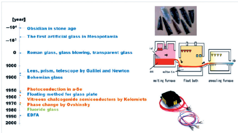
Figure 1 History of glasses, including oxide, chalcogenide, and fluoride. The pictures on the top show obsidian and moldavite, and the below right hand side show, from the top to the bottom , obsidian arrows, a floating method for producing window glasses, and an Er-doped fiber amplifier (EDFA)
