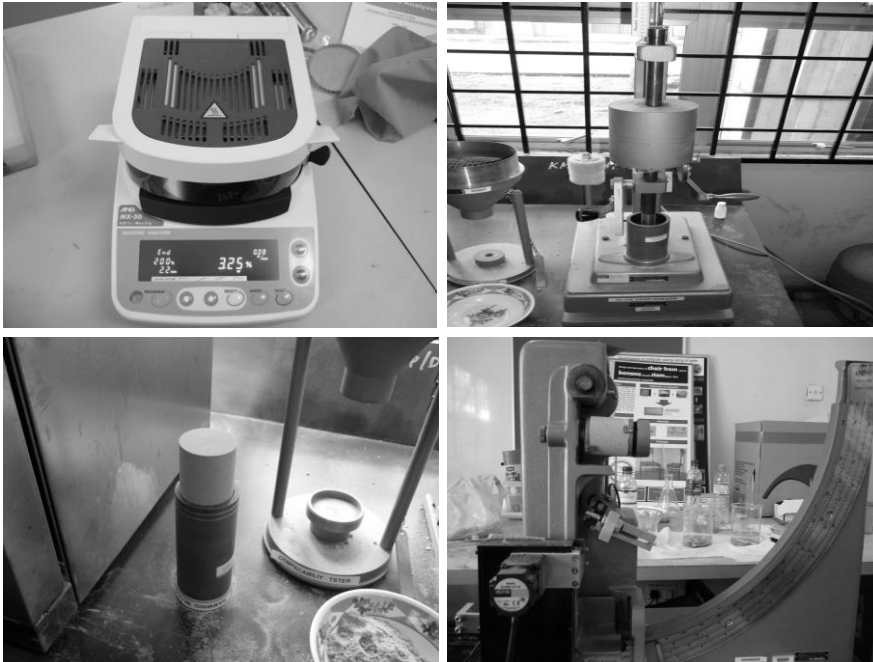
Fig.2: Equipment for foundry sand testing. Moisture analyser(top left), Ridsdale-Dietert metric standard rammer (top right), strip block (bottom left) and Ridsdale-Dietert universal sand strength (bottom right)
