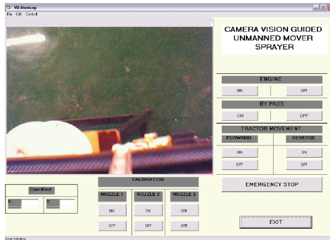
Fig. 3: GUI for controlling the camera vision guided unmanned mover sprayer
