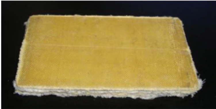
Fig. 1. Final Kevlar29 - ramie composite (the front panel from the TSP)
