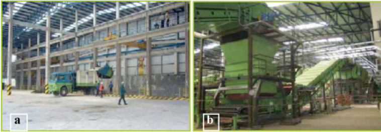
Figure 55 WTE Plant in Semenyih, Malaysia; WTE receiving unit (a) and processing unit (b)
