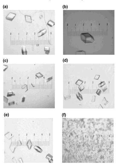
**Figure 33** T1 lipase crystallization at various temperatures: (a) 16 °C, (b) 20 °C, (c) 40 °C, (d) 50 °C, (e) 60 °C, (f) 70 °C. The drop volume consists of 4  $\mu$ L of T1 lipase and 2  $\mu$ L of mother liquor. Scale used was 1:0.1 mm (Source: Leow *et al.*, 2007)
