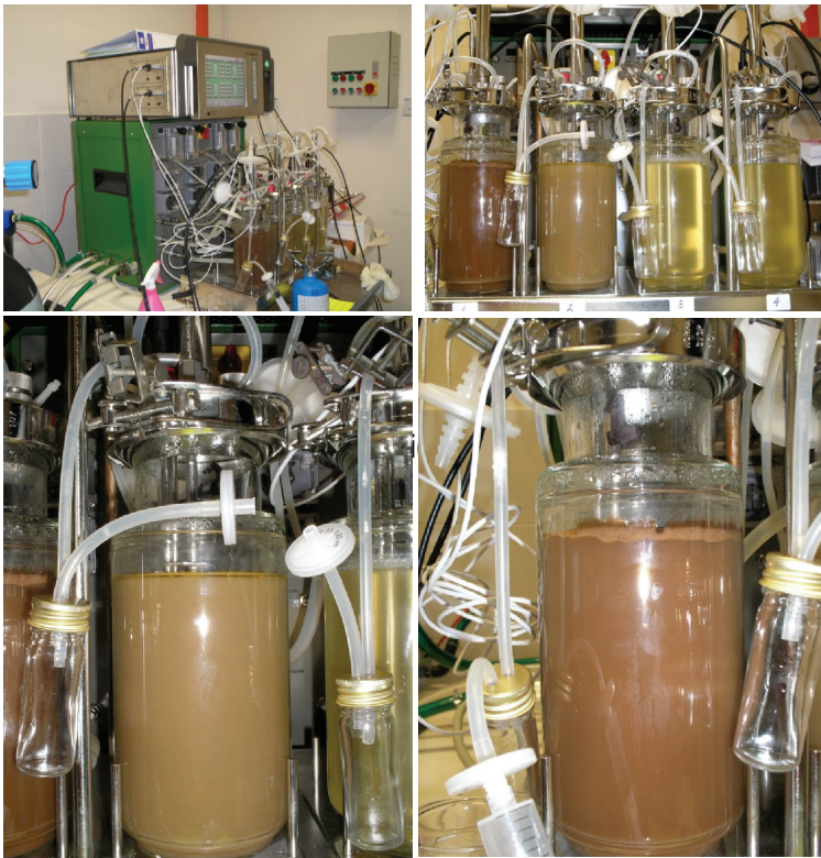
Figure 3 Simulated Human Intestinal Microbial Ecosystem (SHIME) bioreactor system
