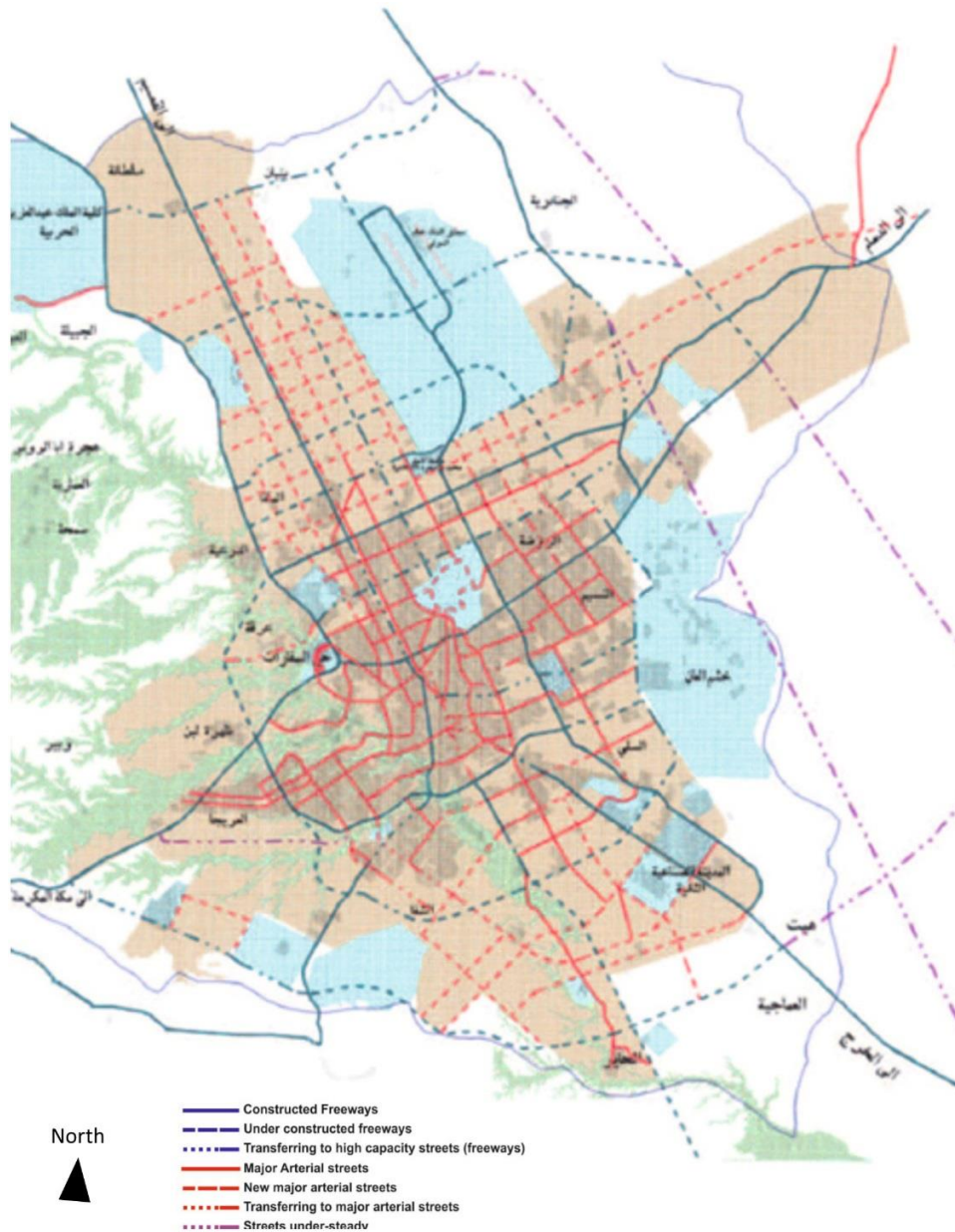
Figure 5-21: The red dotted lines are the new road networks expanding north and east. The transport structure revealed the continuity of the super block 2021 (2x2km).
