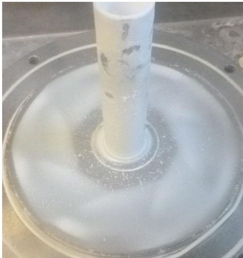
Figure 10.1 Product A Deposition, Top Plate and Vortex Finder
