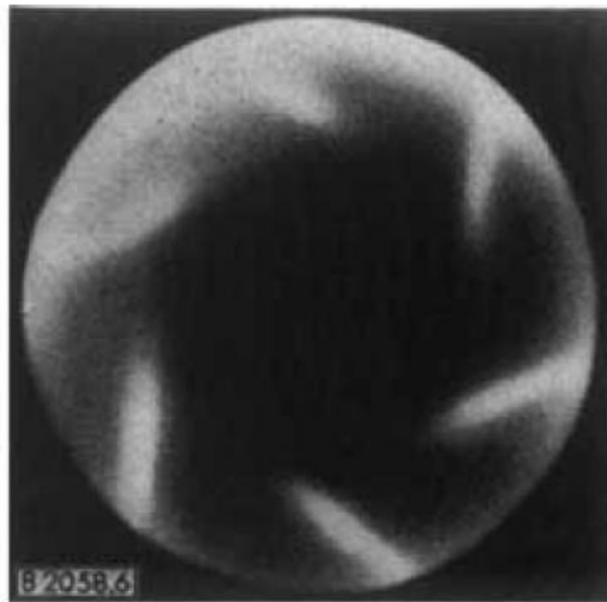
Figure 2.4 Collision Visualisation in a Spiral Jet Mill (Kürten and Rumpf 1966)
