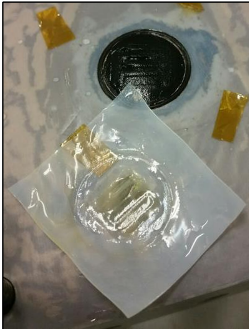
Figure 3.25. Discoloration of the TMA-functionalised AEM exposed to the anode side of the electrolyser setup
