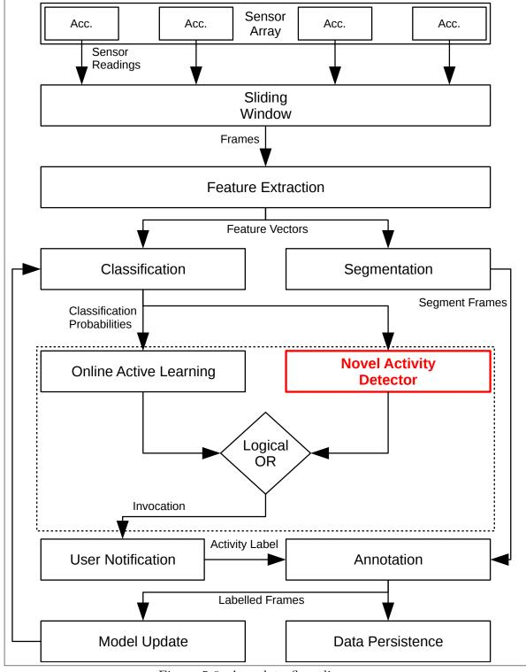
Figure 5.6: App data flow diagram.
