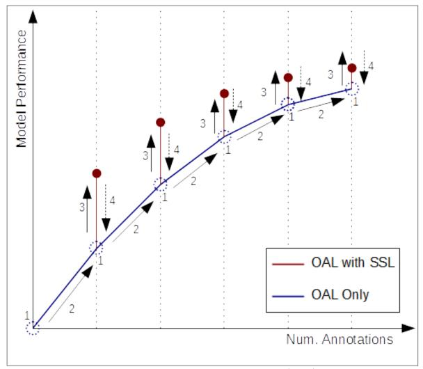
Figure 7.1: Complementing Online Active Learning (OAL) with Other Semi-Supervised Learning (SSL) Methods (Schematic).
