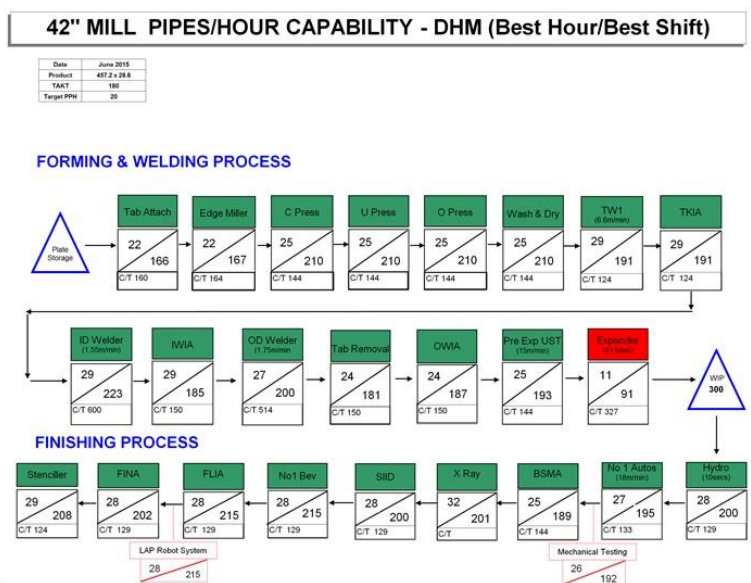
Figure 8.10: Process map illustrating pipe/ hr/ process for 457mm x 28.6mm in 2015.
