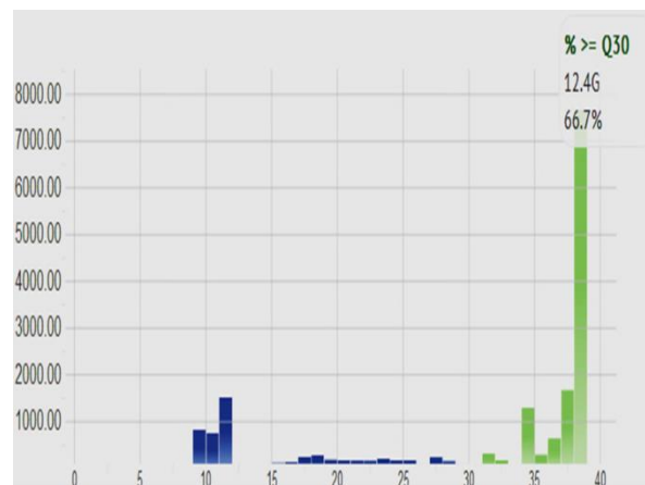
Figure 3-13: Q30 of the sequencing reads generated in MiSeq run. Green bars= number of bases with Q-score >30, Blue bars= number of bases with Q-score<30. Y-axis refers to the number of bases (in millions). X-axis refers to Q-score.
