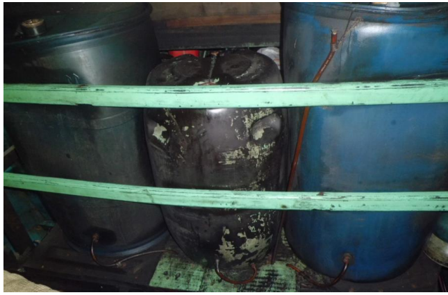
Figure 6.11 Daily fuel tank on-board a traditional fishing vessel in Brondong (Photo by the Author )
