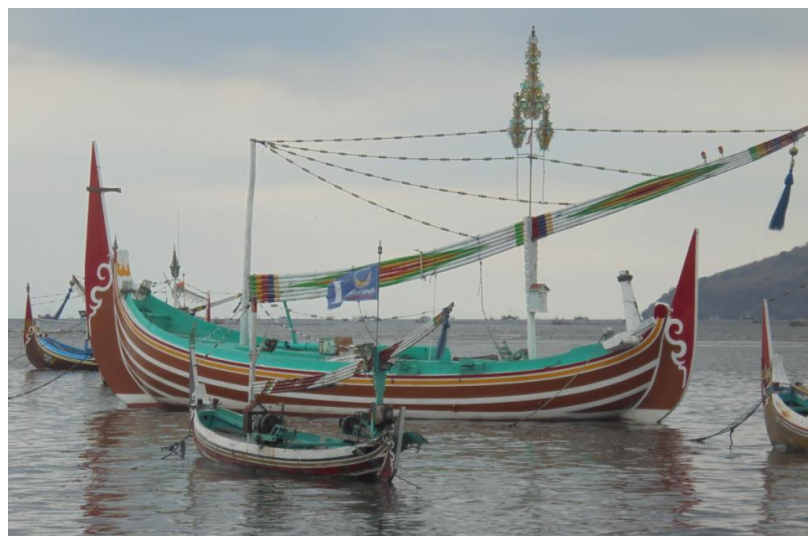
Figure 6.5 Similar shape and proportions of the main dimensions of a large and a small boat in Muncar (Photo by the Author).
