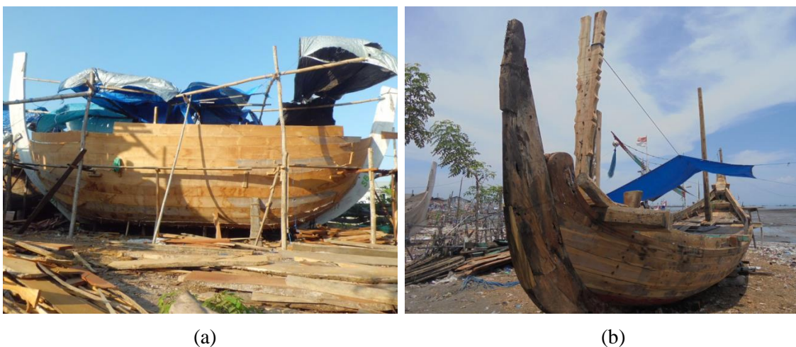
Figure 6.13 Wood used as construction material for fishing boats a) Brondong (Photo by the Author); b) Muncar (Photo by the Author)
