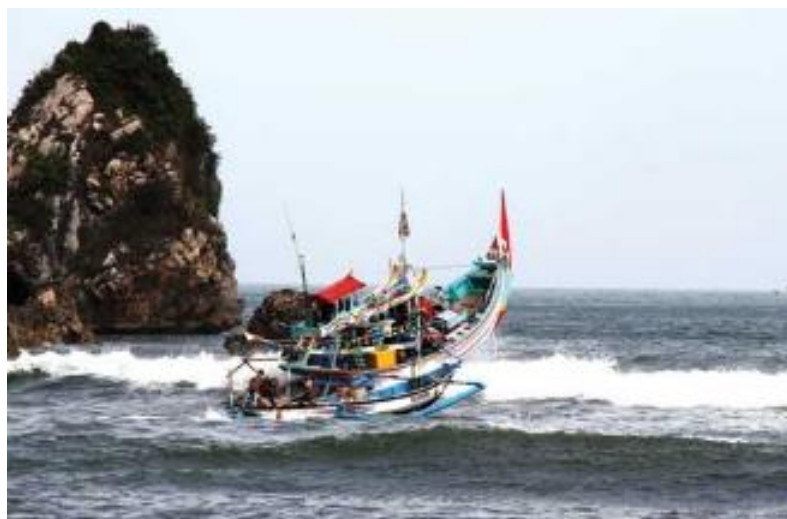
Figure 8.7 The high bow of the Payang boat helps to cope with the surf waves (Source: http://www2.jawapos.com/baca/artikel/18851/sehari-empat-perahu-terbalik-di-plawangan ).
