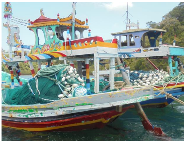
Figure 8.17 Typical wheelhouses for Payang boats in south and east of East Java (Photo by the Author).
