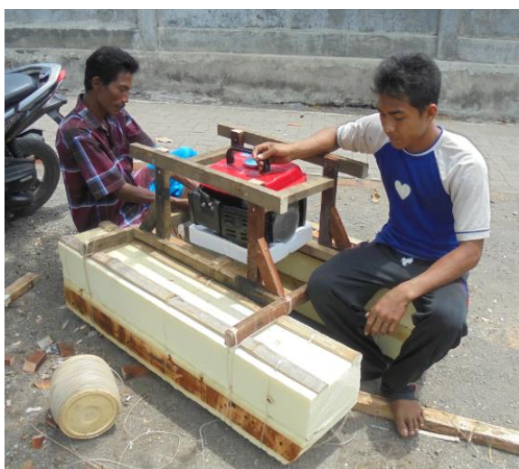
Figure 6.24 A simple polyurethane raft equipped with a genset for FAD in Muncar (Photo by the Author)
