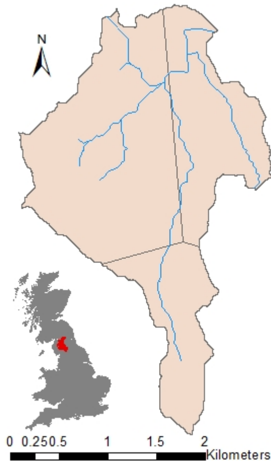
Figure 3-7 Theissen polygons for Morland rainfall weightings used in modelling
