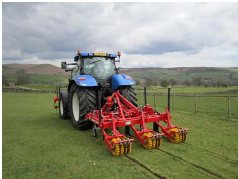
Figure 4-22 Photo of the sward lifting hardware used on the Morland catchment
