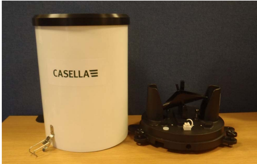
Figure 3-4 Casella tipping bucket rain gauge
