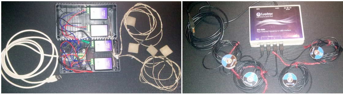
Figure 3.23: Left: The PPS C500, attached to a DLP-IO8 analogue to USB converter. Right: The LoadStar iLoad Mini device. Both devices are capable of measuring force using 4 individual sensors, and reporting the result over USB.
