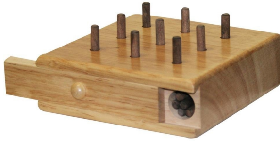
Figure 2.1: An example of a commercially available 9 peg board, used as a measure of motor control; image via Amazon.com
