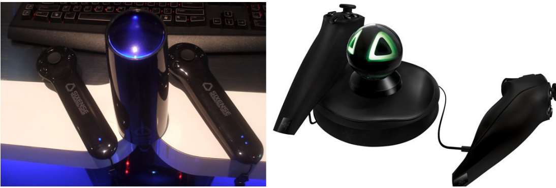
Figure 3.9: Left: The Sixense Truemotion. Right: Razer Hydra. Both devices utilise the Sixense magnetic technology to produce positional and orientation information. Left image from www.cgsociety.org , right image from www.razerzone.com
