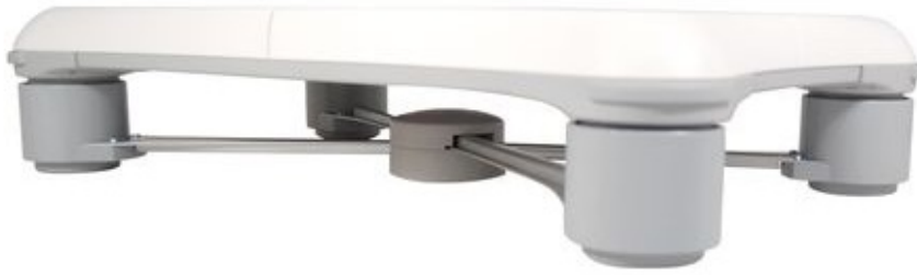
Figure 2.3: The Wii Balance Board device on Step Risers, a combination that could replicate standard motor function assessments such as the Timed Up and Down Stairs Test
