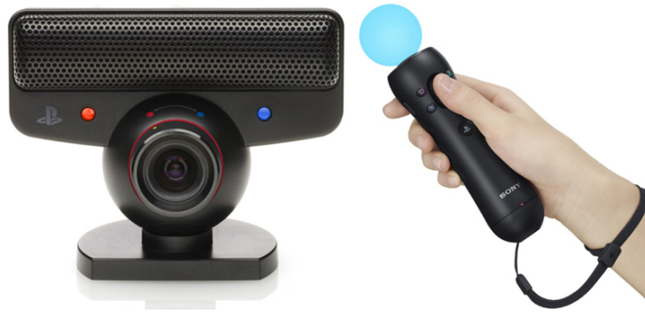
Figure 3.6: Right: The PSEye camera. Left: The PS Move wand. The large coloured orb of the PS Move wand allows image tracking algorithms to be used for accurate positional tracking.
