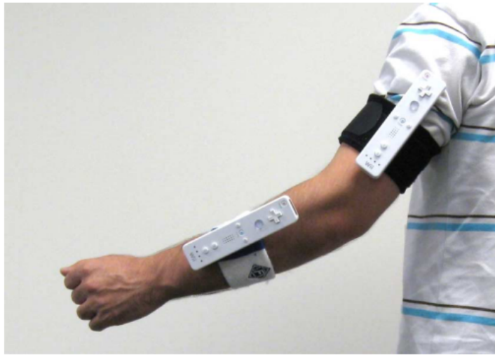
Figure 2.9: Utilising multiple Wii Remotes to determine limb pose by utilising accelerometer data from devices attached to the upper and lower arm, as used in Alankus et al. to control a number of bespoke video games for stroke rehabilitation
