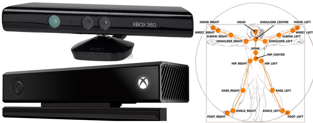
Figure 3.7: Top Left: The Kinect For XBox 360 device. Bottom Left: The Kinect for XBox One. Right: Kinect skeletal tracking joints, determined using a machine learning algorithm within the Kinect software from the colour and depth images. Images from microsoft.com
