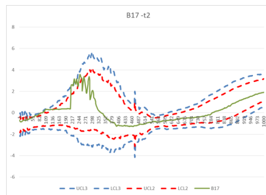
Figure 8-119: B17 Variable-Wise unfolding approach Scores 2 Control limits: 1) UCL3 and LCL3 are upper control limits of + and - 3 standard deviation 2) UCL2 and LCL2 are the lower control limits of + and - 2 standard deviation
