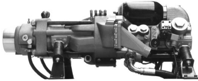
Figure 2.2 Single piston hydraulic free-piston engine from Innas BV [5]
