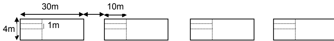
Figure 2.1 Transect layout per site of fish and benthic habitat. Four 10 x 4 m transects were placed inside 30 x 4 m transects. 10 m point intercept transect and 1 x 10 m transect for hole average size and density were also placed inside 30 x 4 m transect.
