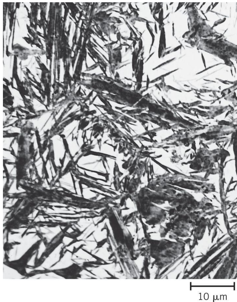
Figure 23. Photomicrograph of the martensitic microstructure. Dark needle shape grains are martensite phase. White regions are austenite phase (Callister, 2015).
