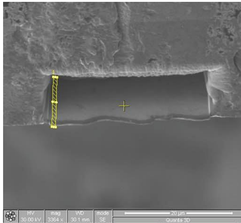
Figure 110. Ion beam was used to mill through the sample to extract the sample with current set to 0.3 nA. The yellow area is the location selected to mill through.
