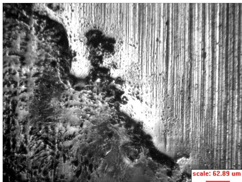
Figure 71. CrN coating containing nanoparticles showing coating failure after the wear test.
