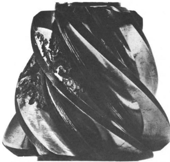
Figure 2. Spalling damage on pinion ( www.orientalmotor.com ).
