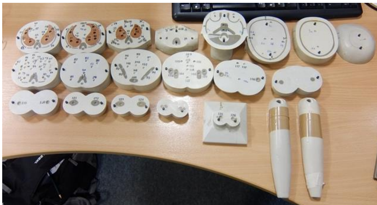
Figure 7.1: Disassembled 1 year ATOM phantom, showing numbered holes in which TLDs can be placed. The arms can also be disassembled. Photo: author
