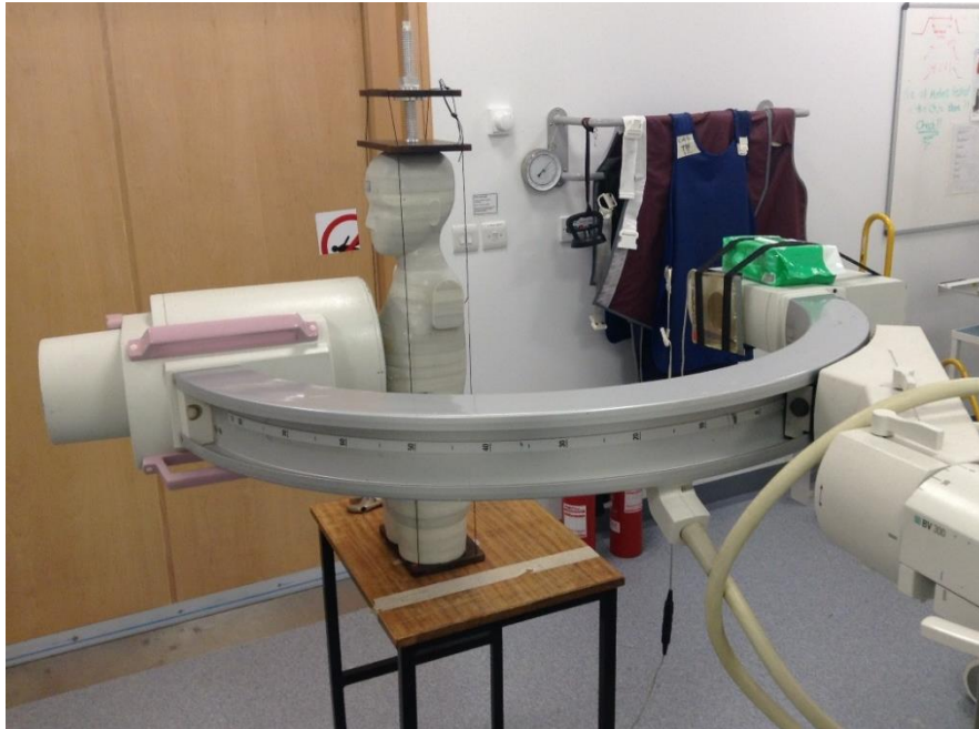
Figure 7.5: Setup for exposures using Philips BV300 mobile C-arm unit. Note the kerma area product meter strapped to the x-ray tube. Photo: author
