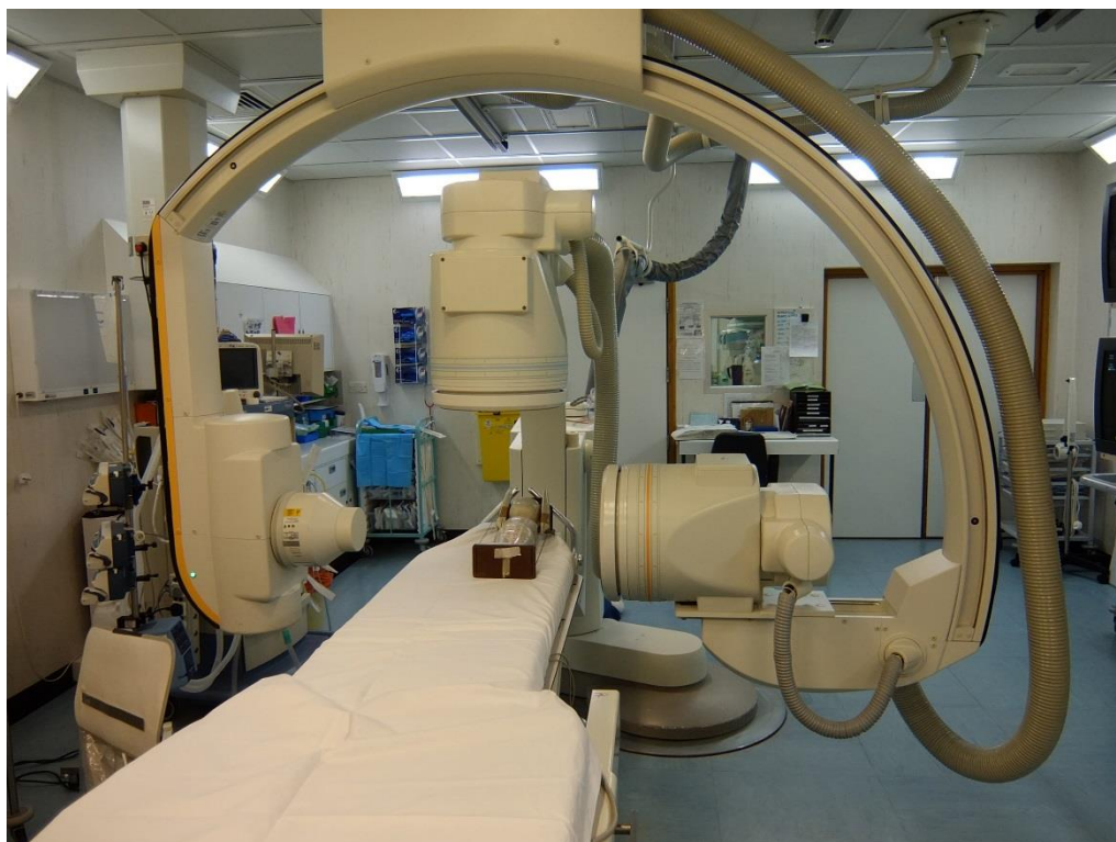
Figure 1.3: A biplane fluoroscopy machine (Siemens Axiom Artis BC). The device pointing in from the left is the lateral x-ray tube, while the device facing this, on the right, is the lateral image intensifier. The frontal x-ray tube is obscured from view, underneath the table. Photo credit: Author
