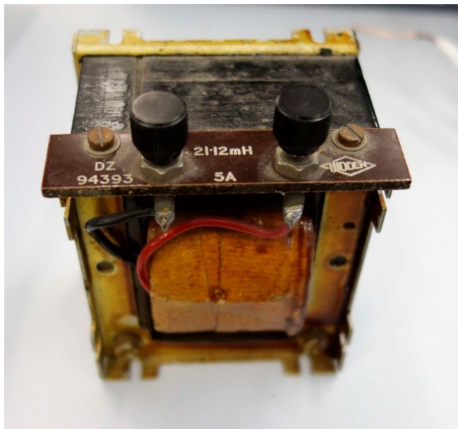
Figure 1-28: E core inductor-21.12 mH
