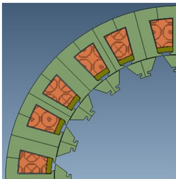
Figure 6-2: MSSRM with magnet moved up the stator
