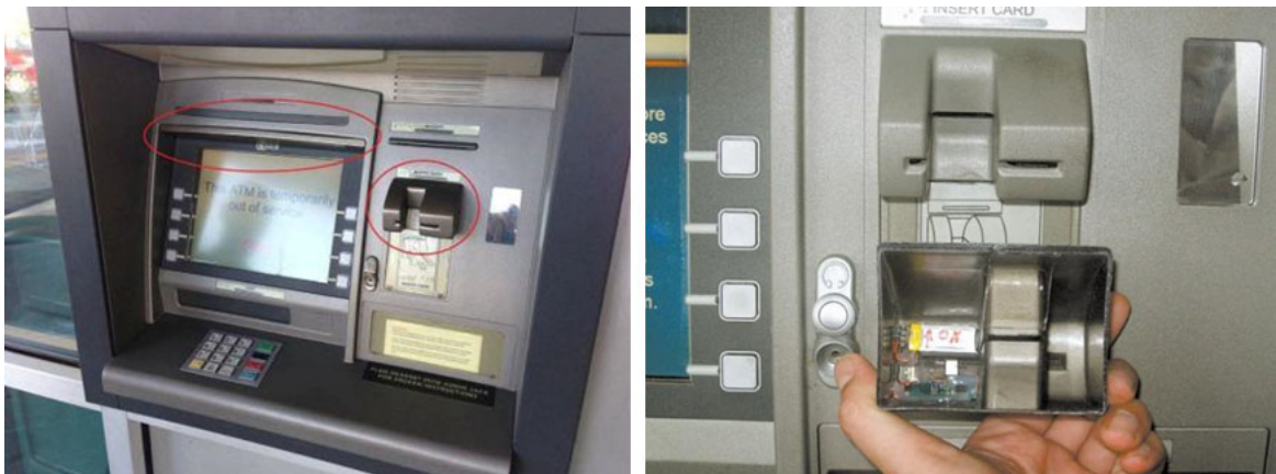
Figure 7 - ATM Magnetic Stripe Skimmer [14]
