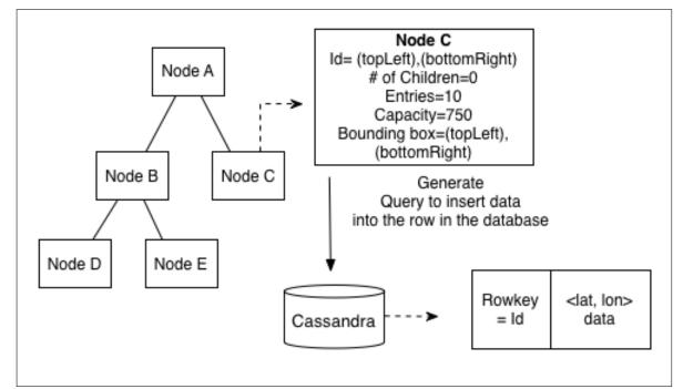
Figure 4.8: The indexing layer converted to Cassandra schema
