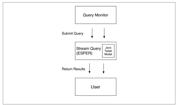
Figure 3.4: Antares: stream querying architecture
