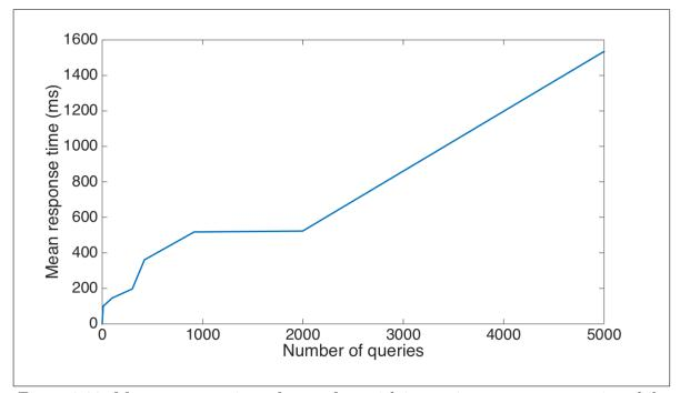
Figure 3.28: Mean response time of query four with increasing concurrent queries while simultaneously inserting to the database
