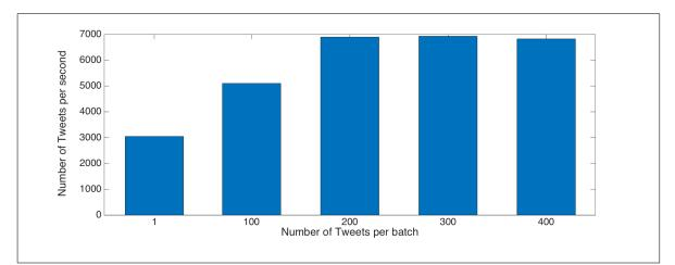
Figure 3.10: Tweets per second written to the *Antares* one-node cluster using increasing batch sizes
