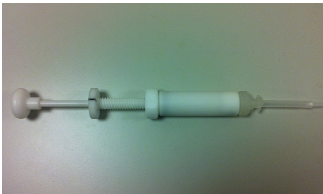
Figure 8: SPE cartridge configuration for succinylation of bound peptides.
