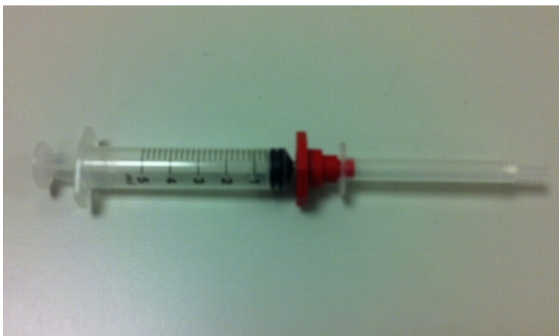
Figure 9: SPE cartridge configuration for guanidination of bound peptides.
