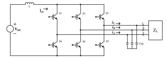
Fig.2 - 11: Schematic of a CSI using IGBT switches
