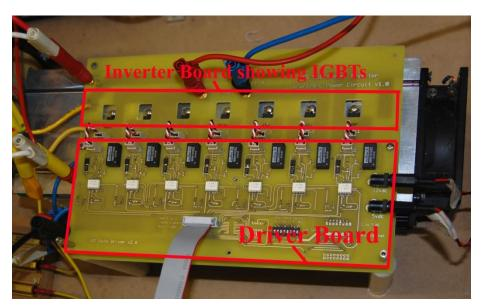
Fig.5 - 3: IGBT driver circuit and the power circuit
