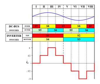
Fig.2 - 29: Topology III Five-level switching sequence
