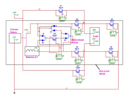
Fig.C.1: Schematic test circuit of the new 5/9-level MCSI
