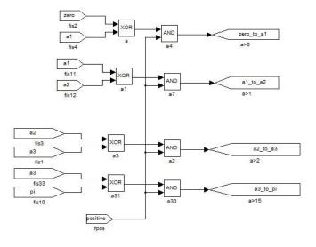
Fig. A.6: The positive cycle block
