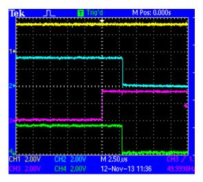
Fig. B.2: Overlapped period of 3us of;(Signal 1: Switch S1a); (Signal 2: Switch S2a)(Signal 3: Switch S1b); (Signal 4: Switch S2b)
