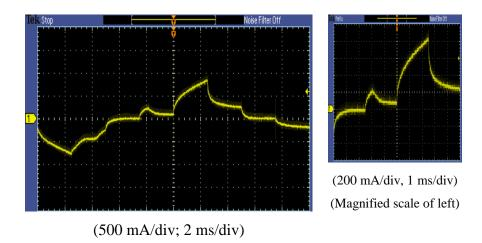
Fig.3 - 15: Five-level output current at high-load condition (with RS technique)
