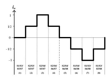
Fig.2 - 19: Five-level CSI switching sequence
