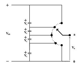
Fig.2 - 4: Multilevel inverter fundamental
