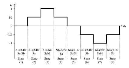
Fig.4 - 4: Five-level CSI switching sequence
