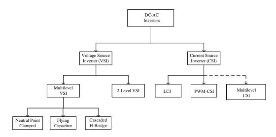
Fig.1 - 1: General Classification of Inverters
