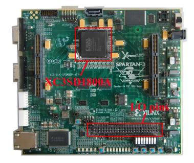
Fig.5 - 6: Spartan 3-A DSP 1800A development board
