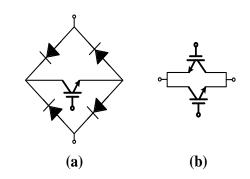
Fig.4 - 1: (a) 1-IGBT with 4-diodes (b) 2-IGBTs in parallel
