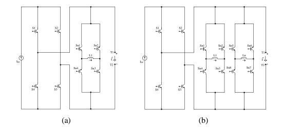
Fig.2 - 32: Topology IV (a) 5-level inverter circuit (b) 9-level inverter circuit
