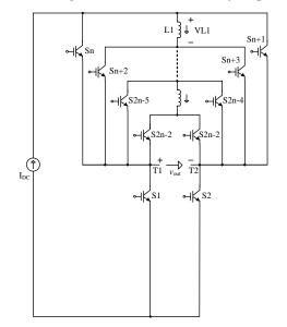
Fig.1 - 3: The generalized structure of Topology II
