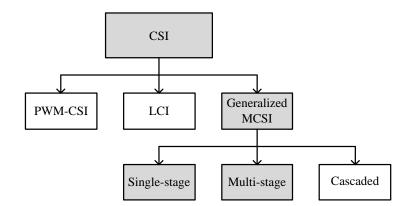
Fig.2 - 12: Generalized MCSI under CSI classification
