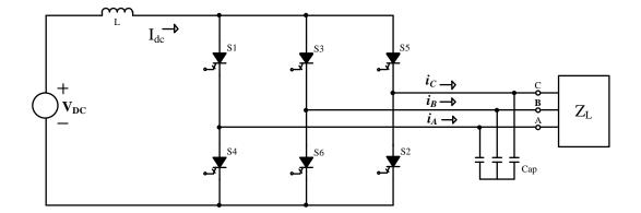
Fig.2 - 9: Schematic of a classical SCR-based CSI
