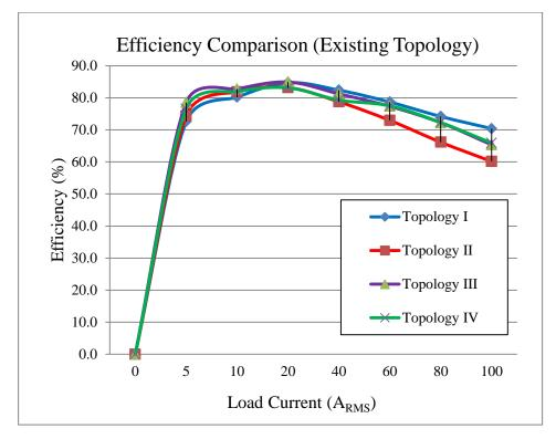
Fig.2 - 36: Efficiency vs. Load Current
