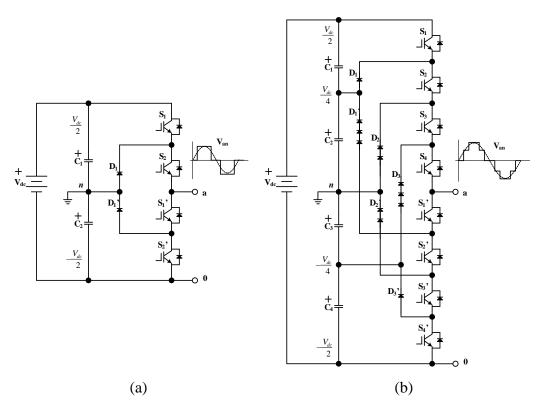
Fig.2 - 5: Diode-clamped inverter (a) three-level (b) five-level
