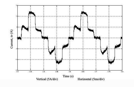
Fig.5 - 9: The five-level output current waveform
