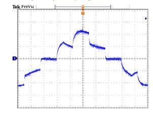
(2 A/div; 2 ms/div) Fig.3 - 14: Typical experimental five-level output current at low-load (with RS technique)
