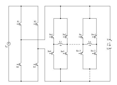
Fig.2 - 31: The generalized structure of the Topology IV
