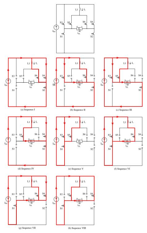
Fig.2 - 26: Single-phase five-level inverter circuit and its corresponding switching sequences (a)-(h)
