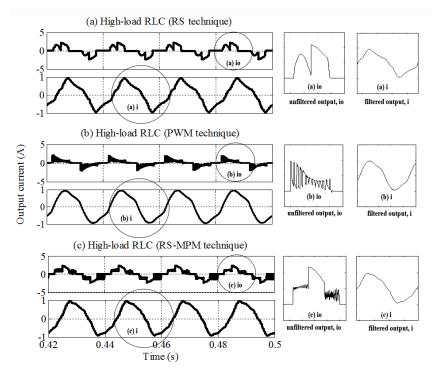
Fig.3 - 12: Simulated output current waveforms (*i*<sub>o</sub> & *i*); high RLC load
