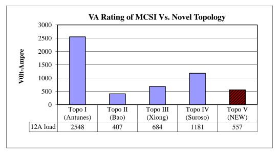
Fig.4 - 17: VA rating of novel topology
