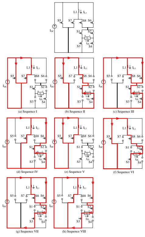
*Fig.2 - 30: Single-phase five-level inverter circuit and its corresponding switching sequences (a)-(h)*
