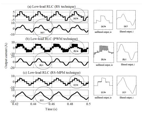
Fig.3 - 10: Simulated output current waveforms (*i*<sub>o</sub> & *i*); low RLC load (a)) *i*<sub>o</sub> & *i* - load current using RS technique
