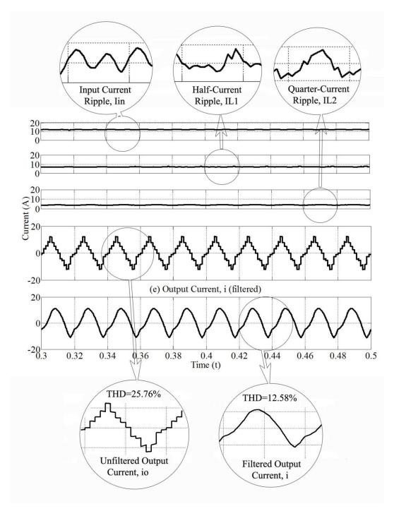
Fig.4 - 13: Nine-level CSI with equal switching angles
