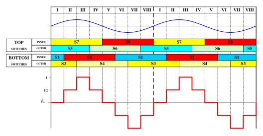
Fig.2 - 21: Five-level symmetric switching sequence
