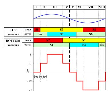
Fig.2 - 22: Five-level asymmetric switching sequence
