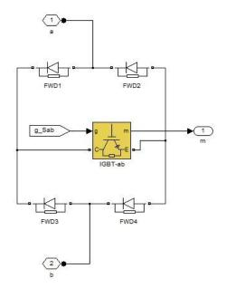
Fig. A.2: The bidirectional IGBT switch
