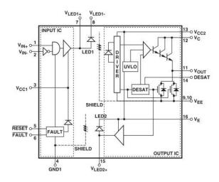
Fig.C.3: HCPL-316J IC inside components [99]
