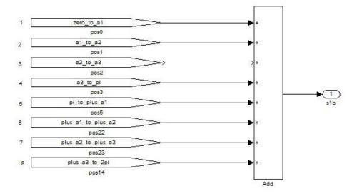
Fig. A.16: The logic signals of the switch S1b
