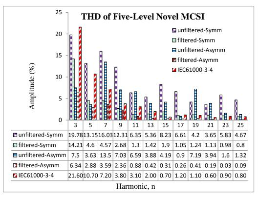
Fig.4 - 15: Current harmonic contents of the novel five-level topology
