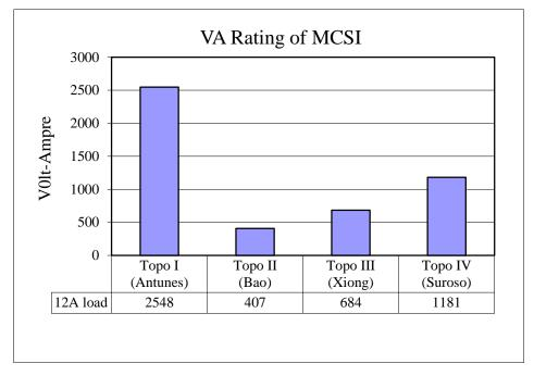
Fig.2 - 35: Volt-Ampere (VA) comparison
