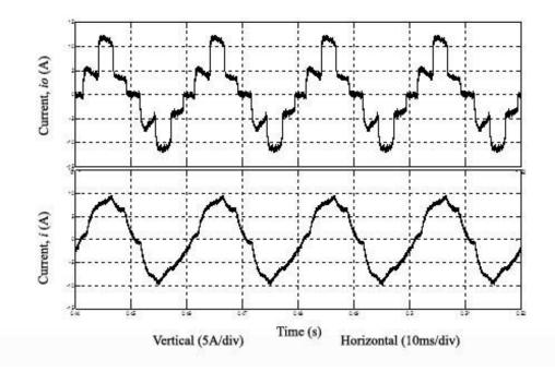
Fig.5 - 10: The output current before and after filtering
