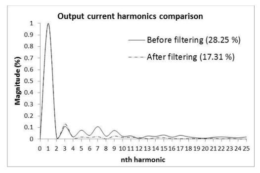
Fig.5 - 11: Harmonics comparison before and after filtering
