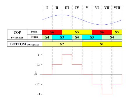
Fig.2 - 25: Topology II five-level switching sequence
