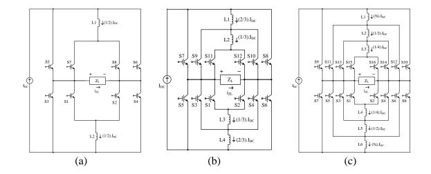
Fig.2 - 18: Topology I (a) 5-level (b) 7-level (c) 9-level
