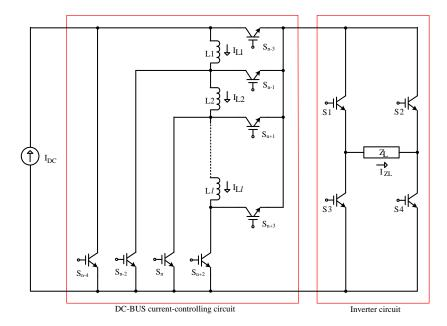
Fig.1 - 4: Generalized structure of Topology III
