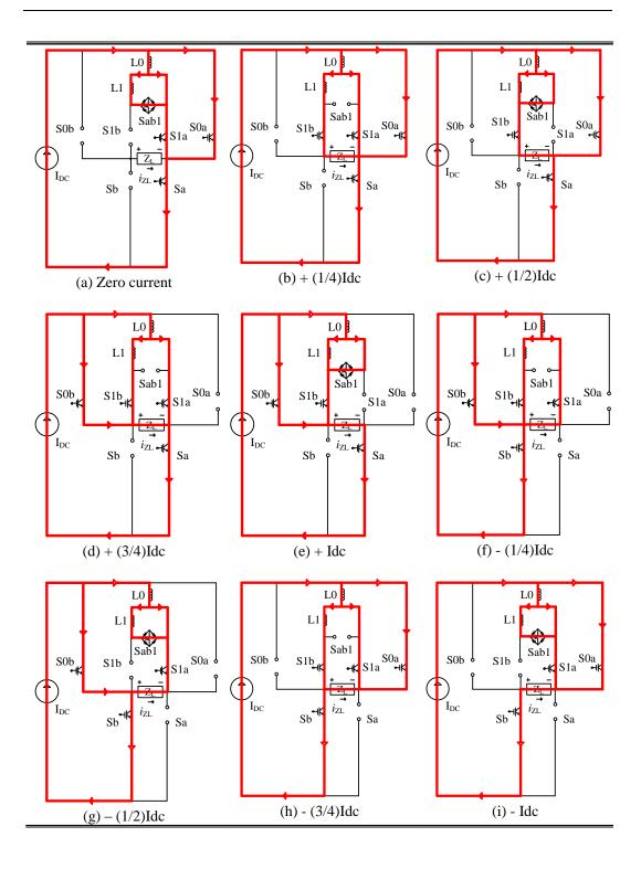
Fig.4 - 7: Load current path of the nine-level CSI
