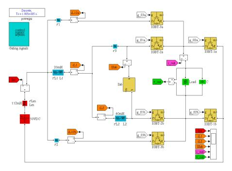
Fig.4 - 9: Matlab/Simulink model of the novel nine-level CSI
