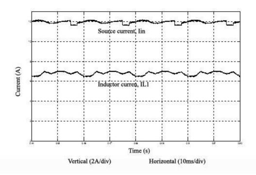
Fig.5 - 8: The source current and inductor current waveforms
