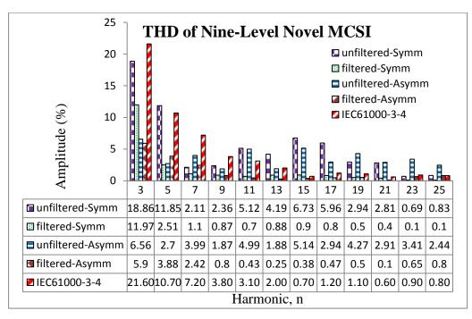
Fig.4 - 16: Current harmonic contents of the novel nine-level topology
