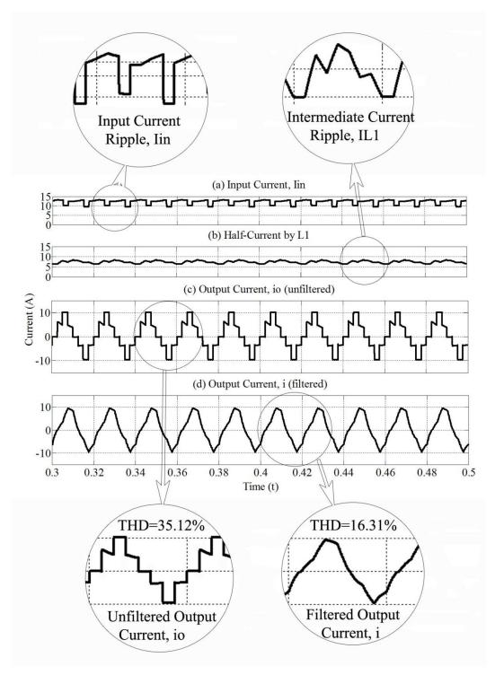
Fig.4 - 11: Five-Level CSI with equal switching angles
