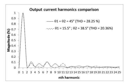
Fig.5 - 16: Harmonic contents improved at specific switching angles,  $\theta$
