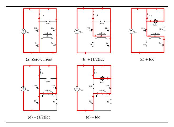
Fig.4 - 5: Load current path of the five-level CSI
