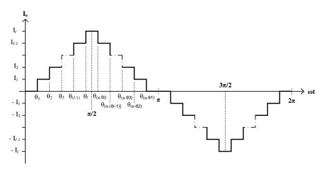
Fig.2 - 2: Output current waveform of a general single-source MCSI
