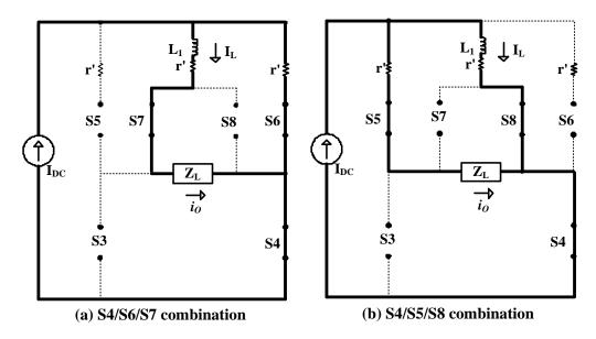
Fig.3 - 7: Half-current redundant switching states
