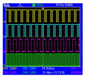
Fig. B.4: Logic signals in 25ms of; (Signal 1: Switch S1a); (Signal 2: Switch S2a) (Signal 3: Switch S1b); (Signal 4: Switch S2b)
