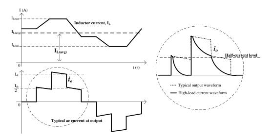
Fig.3 - 6: Typical average inductor current (top, left); the respective five-level output current waveform (bottom, left) and its comparison to the high-load current condition (as highlighted on the right).
