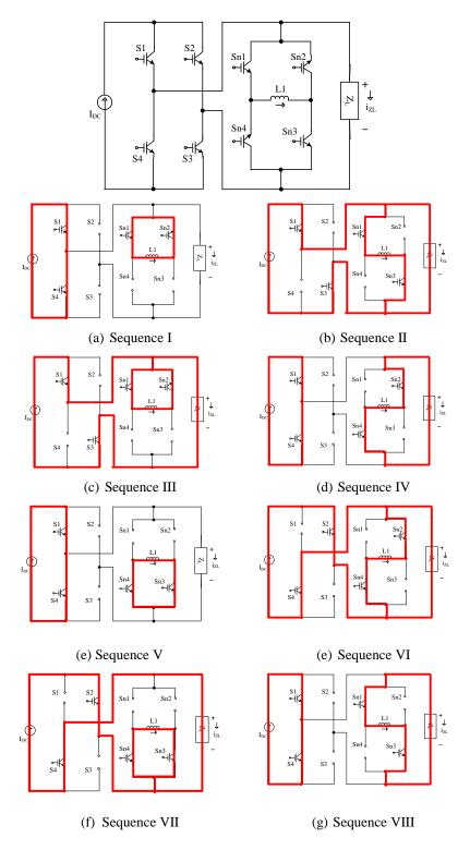
*Fig.2 - 34: Single-phase five-level inverter circuit and its corresponding switching sequences (a)-(h)*
