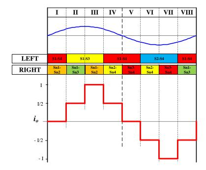
Fig.2 - 33: Topology IV five-level switching sequence
