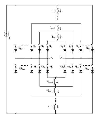
Fig.2 - 16: Final MCSI circuit
