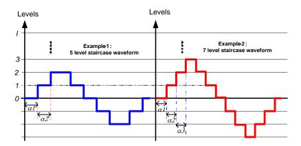
Fig.2 - 1: Converter output level determination
