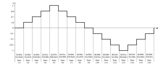
Fig.4 - 6: Nine-level CSI switching sequence
