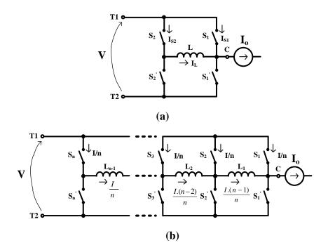
Fig.2 - 14: The original generic cell; (a) single-cell (b) multiple-cells
