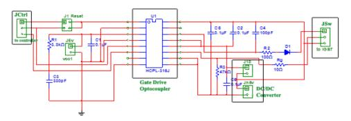
Fig.C.4: Schematic for the gate driver circuit
