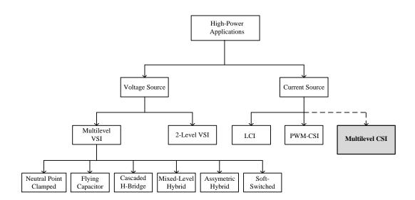
Fig.2 - 3: Classification of converters for high-power applications
