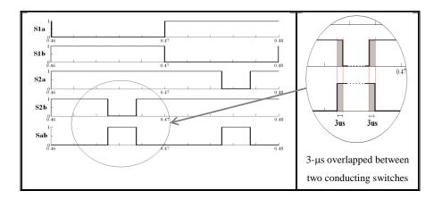
Fig.4 - 10: Five-level CSI gate signals with overlapping periods highlighted
