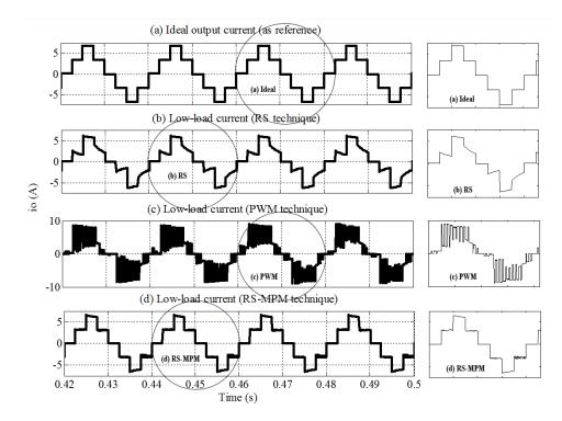
Fig.3 - 9: Simulated output current waveforms; low resistive load (from the top: ideal, RS, PWM and RS-MPM)
