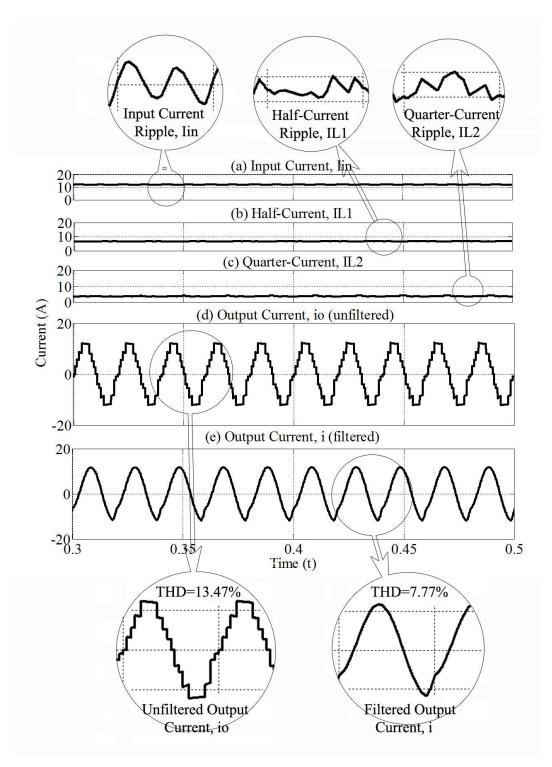
Fig.4 - 14: Nine-level CSI with variable switching angles
