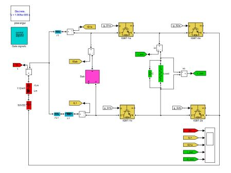
Fig.4 - 8: Matlab/Simulink model of the novel five-level CSI
