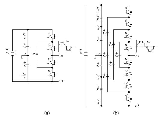
Fig.2 - 6: Capacitor-clamped inverter (a) three-level (b) five-level
