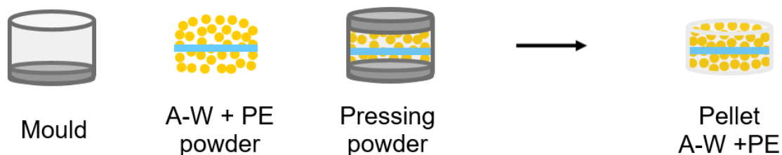
Figure 3-9: A-W compacted powder with polymeric filament.
