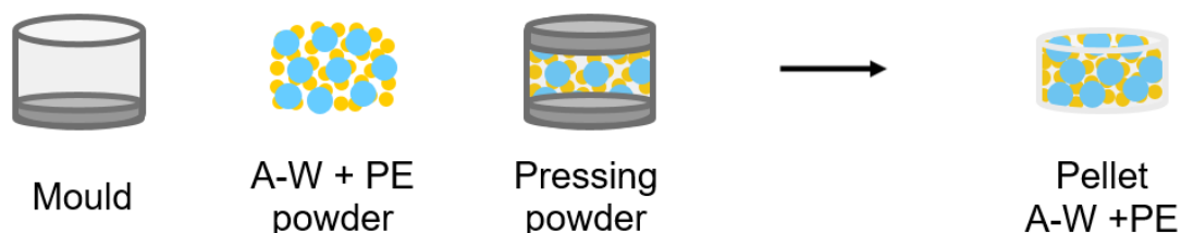
Figure 3-8: A-W compacted powder with PE particles
