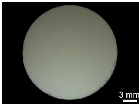
Figure 3-14: Morphology of sintered pellet scaffold fabricated with pure A-W. Representative bright field image of pellet scaffold. Scale bars, 3mm. The image A was acquired using lens 0.5 at magnification 3x.
