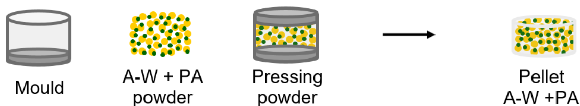
Figure 3-7: A-W compacted powder with PA particles
