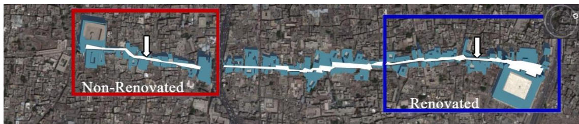
Figure 5-21 The two modelling domains and the two measurement points which are the same receptors in ENVI-met
