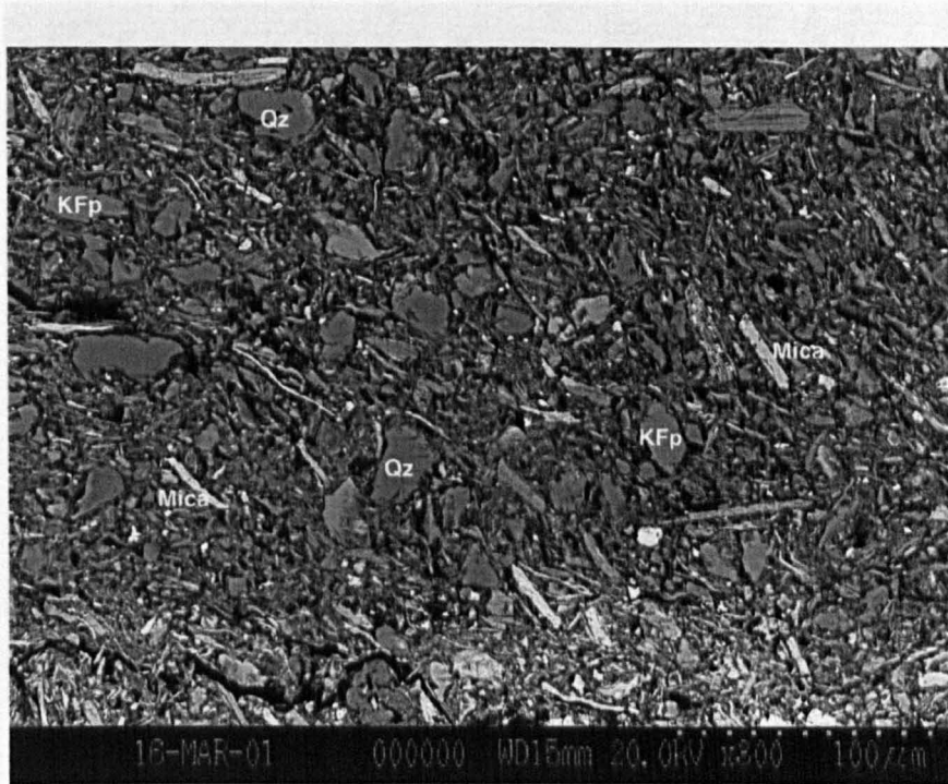
Fig. 97 BSEM image of a shallow (1270mbsf), fine silt (35% <math><2\mu\text{m}</math>) sample from the Bay of Bengal. The overall alignment of the phyllosilicates in this silty matrix is relatively weak (3.03m.r.d. for illite/mica). Qz = quartz; KFp = K-Feldspar.
