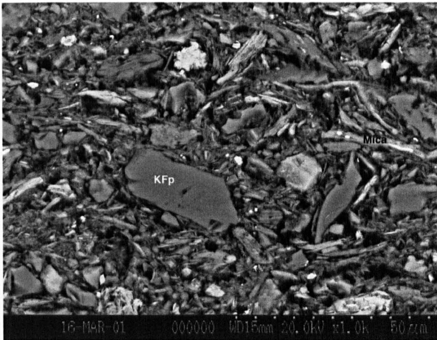
Fig. 98 BSEM image of the same Bay of Bengal sample as in Fig. 97. This magnification illustrates the lack of preferred orientation for most of the fine-grained ( <5\mu\text{m} ) mica particles.
