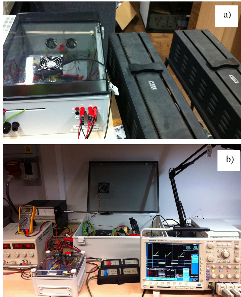
Figure 3.2: Test setup for converter evaluation based on different semiconductor technologies (a) and (b)
