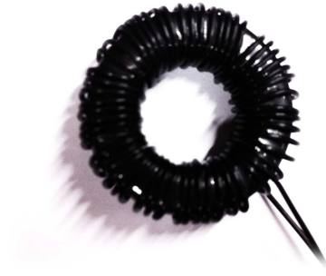
Figure 5.25: The coupled inductor wound on a high temperature toroid
