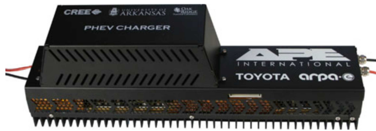
Figure 2.16: Full charger system hardware [100]
